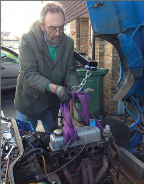
Picture 5: Spitfire 1500 engine lifting (photo by Antony Wootton)
