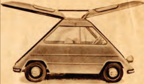
The Dornier Delta four-wheel cabin scooter is referred to on this page. Passengers sit back to back with maximum leg room
