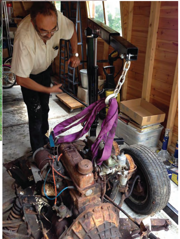
Photo 4: Spitfire 4 engine lifting (photo by Glenn Howard)
