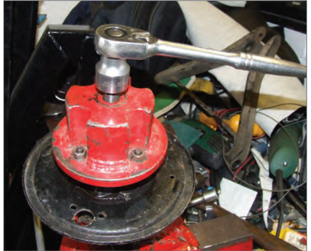
Picture 2: Hub puller in action
